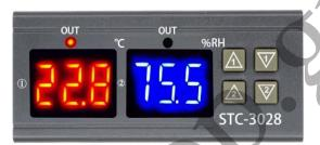
Long press  $\underline{\Lambda}$  3 seconds, the starting temperature value flashes (default 20  $^{\circ}$  C) Press the plus or minus button to adjust, long press  $\underline{\nabla}$  3 seconds, stop the temperature value flash (default 30  $^{\circ}$  C) press the plus or minus button to adjust.
